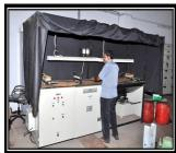
MAGNETIC CRACK DETECTION MACHINE
