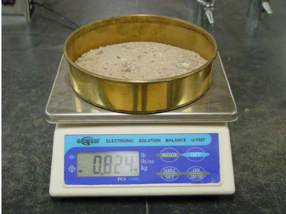
Fig: Illustrates Sieve Analysis test procedure
