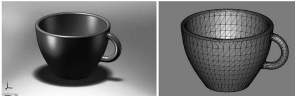
A CAD model on the left converted into STL format on the right
