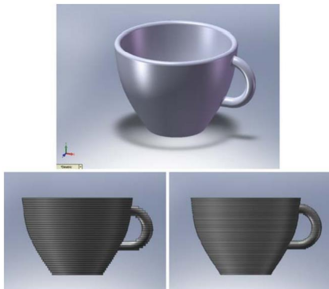
CAD image of a teacup with further images showing the effects of building using different layer thicknesses
