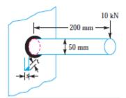
13. A rectangular cross-section bar is welded to a support by means of fillet weld as shown in Fig. Determine the size of the welds, if the permissible shear stress in the weld is limited to 75 MPa.
