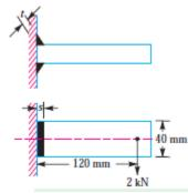
12. A 50 mm diameter solid shaft is welded to a flat plate as shown in Fig. If the size of the weld is 15 mm, find the maximum normal and shear stress in the weld.
