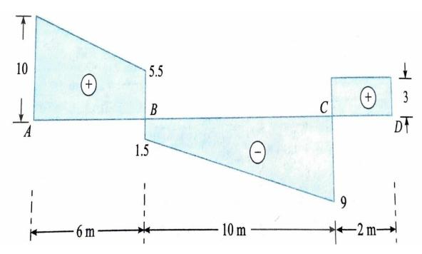
Duduce directly from the shear force diagram ,(a) loading on the beam, (b) bending moment At 2 m intervals along the beam and (c) position of the second support. Also draw bending moment diagram for the beam and indicate the position and magnitude of the maximum value on it.
