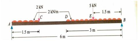
Draw the shear force and bending moment diagram for the beam.
