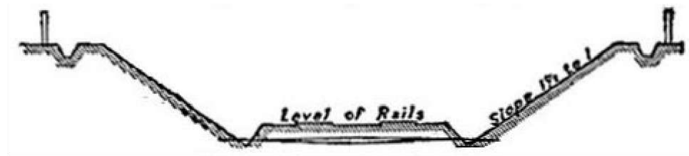
Typical Section of Railway in Cutting.
