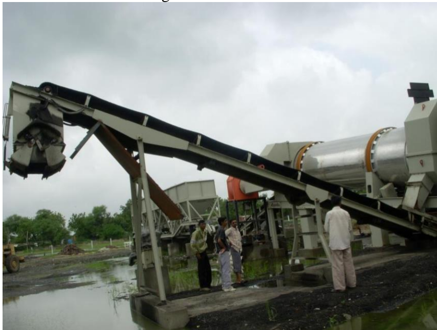
Fig. Load Out Conveyor
