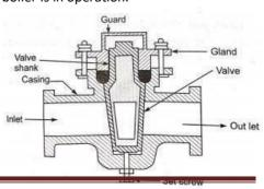
the corresponding hole in the casing. The plug valve has a hole, which when brought in linewith the hole in the casing, by rotating the plug, causes the water to flow out of the boiler.
