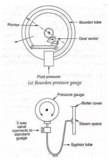
The siphon tube connects the steam space of the boiler to the Bourdon gauge is filled with water in order to avoid the effect of high temperature steam on the gauge components. Thesteam pressure is transferred by water to the Bourdon pressure gauge.
