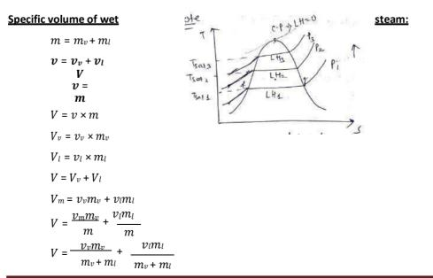
$V = v_{v}x + v(1 - x)$  $V = v_{v}x + v_{l} - xv_{l}$  $V = v_{l} + x(v_{v} - v_{l})$
